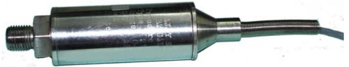
“AJAY SENSORS” Pressure Transmitter, Type 210 - g series utilize four temperature matched foil strain Gauges within a robust stainless steel construction, providing a highly stable bridge with precise pressure conversion performance and excellent resistance to oxidation, chemical and metallurgical changes.
