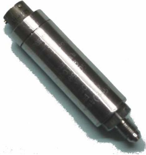
“AJAY SENSORS” Pressure Transducer, Type PT 209 A - g/abs. series is based on a high performance sensor developed specifically for industrial and process applications. Uses 316 stainless steel diaphragm and stainless steel body, which is compatible with most fluid and gaseous pressure media.
