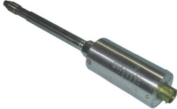
“AJAY SENSORS” Melt Pressure Transducer, Type PT 112 series is based on a high performance sensor developed specifically for industrial and process applications. Uses stainless steel diaphragm and stainless steel body, which is compatible with most fluid and gaseous pressure media.
